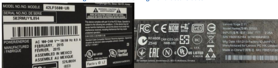
Figure 2. Labels showing manufacture date
